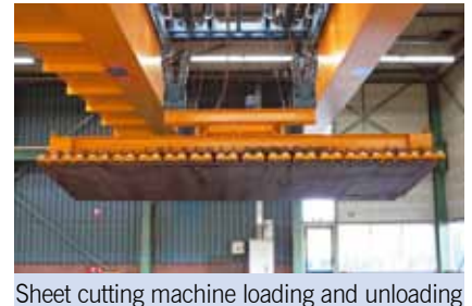
Sheet cutting machine loading and unloading
