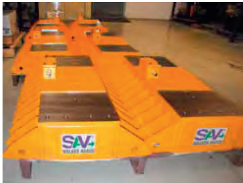
Special purpose built magnets for the alignment of steel sheet in the rolling mill before the guillotine.
