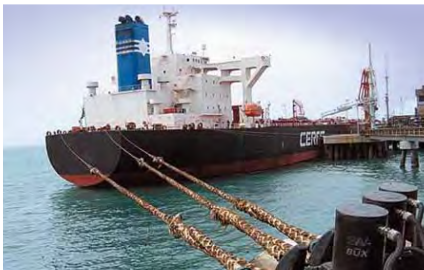
Special electromagnetic solenoids in the harbour. In case of emergency these solenoids actuate quick release mooring hooks.
