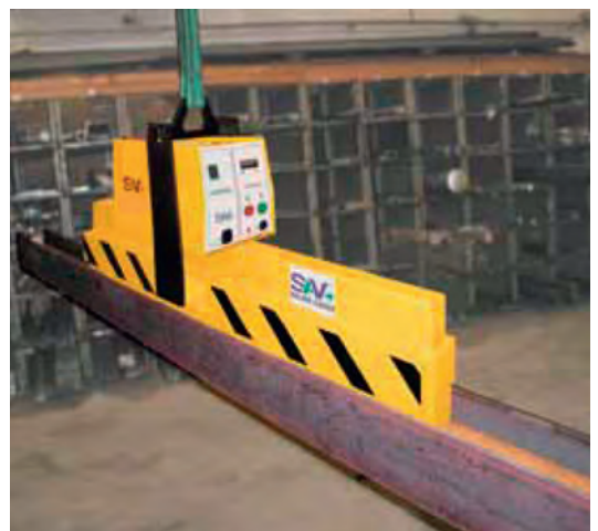
Handling of a cut-off beam at a sawing machine
