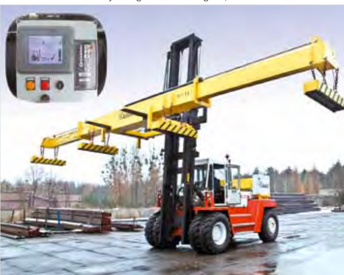
Telescopic beam with magnets on a fork lift truck. The power to the magnets is provided by a generator mounted on the truck
