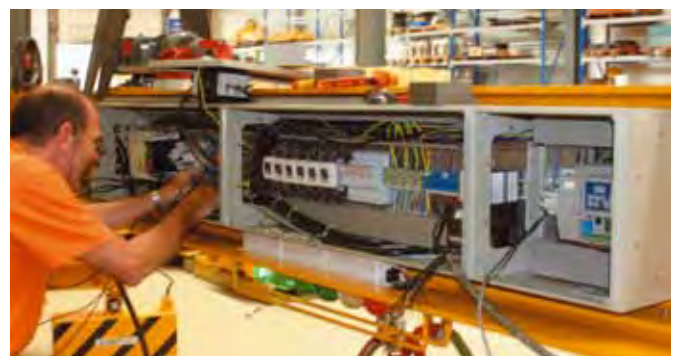
The control cabinets can be integrated into the beam on request.
