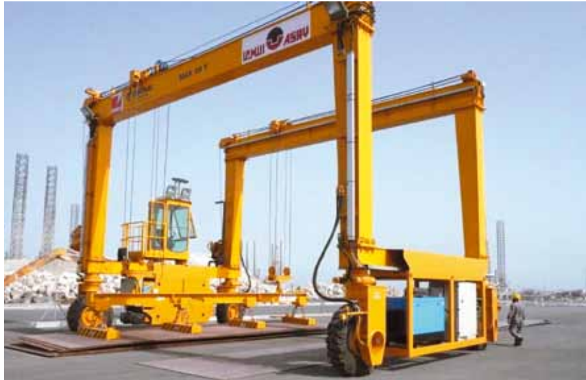
Beam with magnets on a mobile gantry crane.
