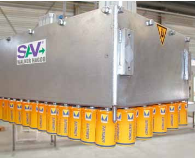
Pneumatically operated permanent palletizer magnet for the palletizing of batteries. The entire contact surface is magnetic.
