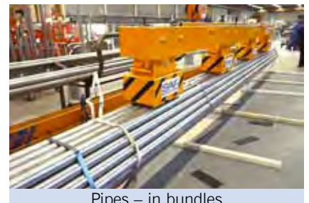
Pipes – in bundles
