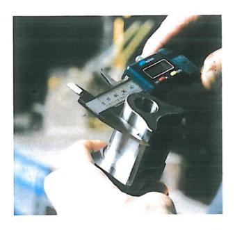
First aid fast! The Coolant Audit S provides an initial and immediate way of determining lubricoolant oversupply and undersupply of a machining site (all production processes). Flow rates and supply pressures are measured on a machine tool for a selected production scenario and the geometries of the process-relevant lubricoolant supply nozzles are recorded.
