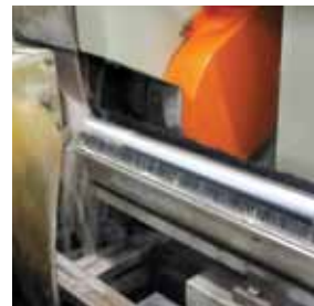
To obtain a very low surface finish (under 0.5) and create a mirror effect shine use cork and silicon carbide in P400 to P800 grits.
