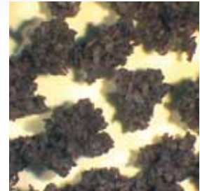
Small aluminium oxide particles are bonded together to create an aggregate grit.
